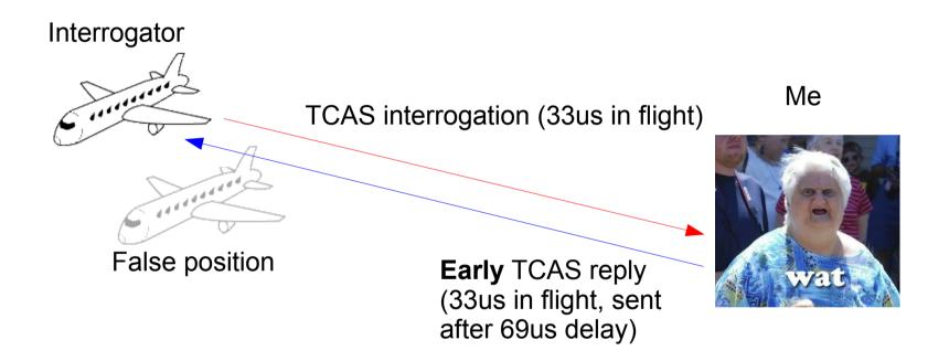
Real distance from transponder: 10km Time lag: 66us + 69us calculated delay
