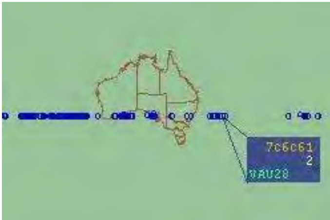
Figure 1 - Track Jumping problem with TPR901
