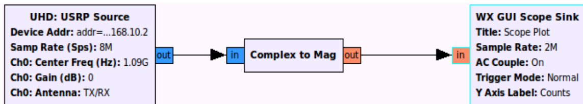
Figure 23 - GRC view of the ADS-B troubleshooting application
