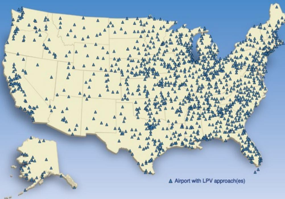
The FAA continues to deploy procedures that improve access to many general aviation airports in almost all weather conditions. Localizer Performance with Vertical Guidance (LPV) are precision GPS approaches, enhanced by Wide Area Augmentation System signals, that provide vertical guidance as low as 200-250 feet above the runway for equipped aircraft.
