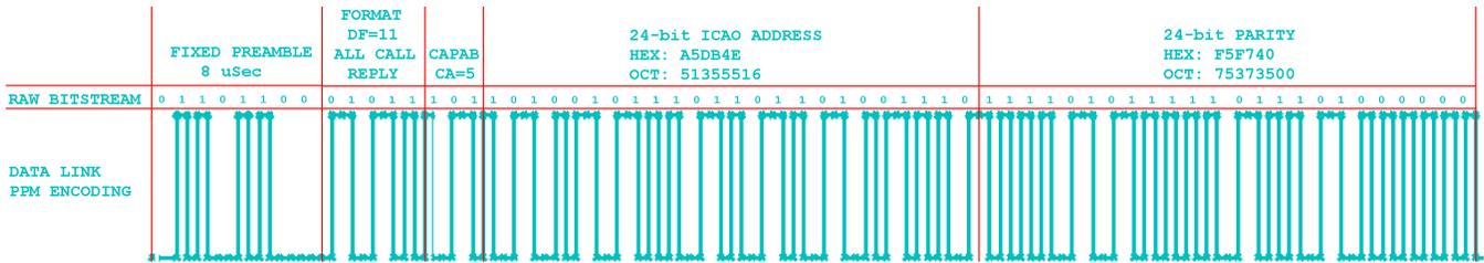
Figure 2. PPM-encoded ADS-B 56 bit sample frame.
