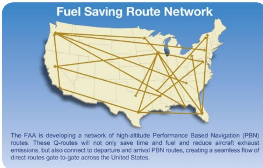
The ongoing Q-route implementation plan will bring end-to-end PBN functionality to the NAS by providing seamless flight paths between departure and arrival RNAV routes. We have identified 12 Q-route network projects. Each project will have multiple Q-routes spanning multiple air route traffic control centers. We will further optimize the network as needed to generate additional user benefits.
